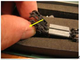
Now slide the truck side frame over the wheels with pickup. Using your right hand while holding the pickups in position with your other hand.
