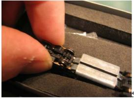
Double check that the pickup contacts are in the right position.
