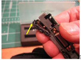
Lock the truck side frame in position with the remaining part of the coupler box.
