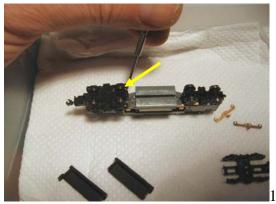
Removing the truck sides.
